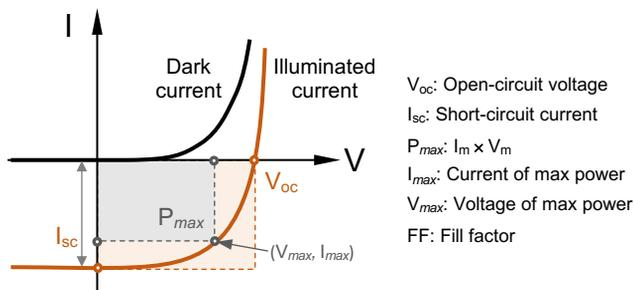
Figure 1. Dark and illuminated I-V curves of a solar cell.
