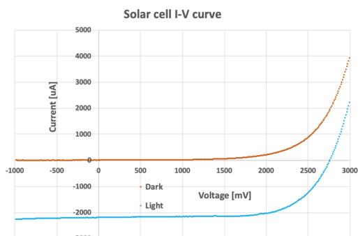
Figure 4. Dark (orange) and light (blue) I-V curves of a solar cell using Elite-EDC.
