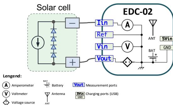
Figure 2. Equivalent circuit of an Elite-EDC connect to a solar cell for I-V characterization.
