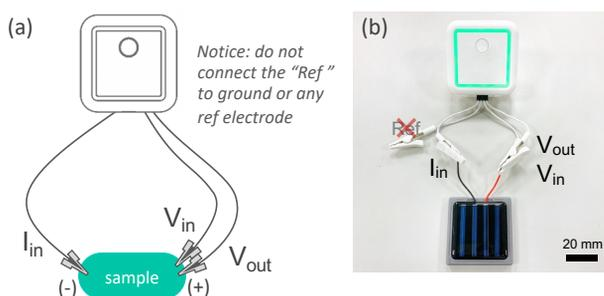
Figure 3. Schematic illustration (a) and photograph (b) of measuring I-V characteristics of solar cells using Elite-EDC. (solar cell part No: 109985, Centenary).
